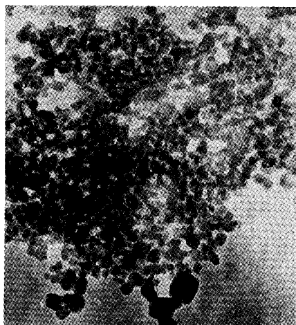
Fig. 1 The TEM photograph of CuHCF nanoparticles. Scale bar: 100 nm.
